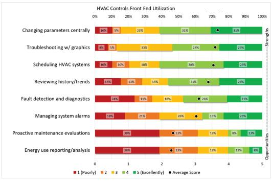
Figure B-2. Building automation front-end feature utilization best practices.
