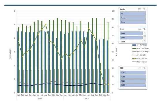
Figure 4. Army Barracks Electric EUI Apparently 7 X Other Services.
